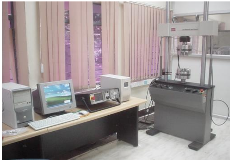
Figure 15 100-kN MTS servo hydraulic test system
