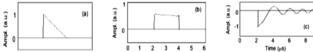
Figure 9 Displacement profiles generated by a 2 \mu s toneburst. (a) Displacement pulse obtained for \beta > 0 . (b) Displacement pulse obtained for \beta > 0 . (c) Displacement pulse profile obtained oscillatory tail for a dispersive material with \beta < 0
