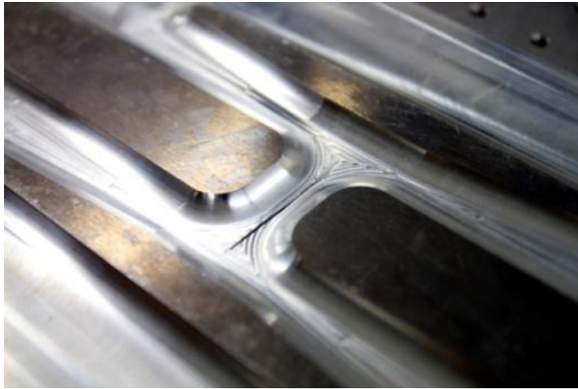
Figure 5.1: Fatigue critical location on the F111 underwing skin
