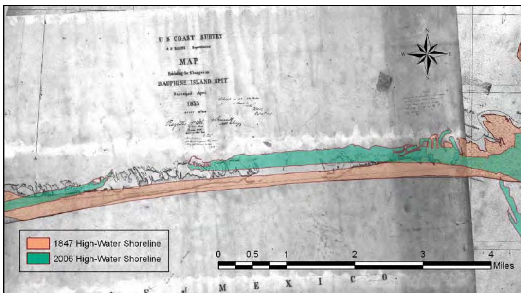
Figure 2-26. 2006 shoreline overlying the 1847 shoreline and the breached area in 1853, illustrating barrier rollover and breaching on central Dauphin Island.
