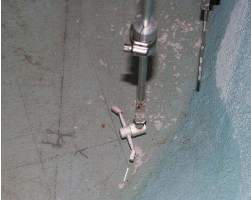
Figure 21. Acoustic Doppler velocimeter probe head.
