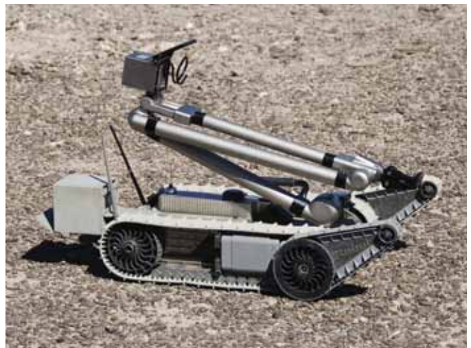
Small unmanned systems provide opportunities to supply organic, stand-in sensing capabilities to small units. The Laboratory is working with industry to integrate Laboratory-developed sensors on robots, such as the Packbot pictured above.
