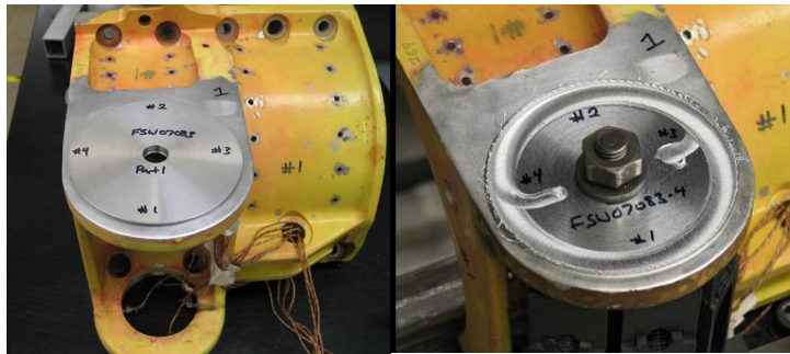
Figure 14: Dry-fit of Repair Plug (left) and Post Weld Repair (right)
