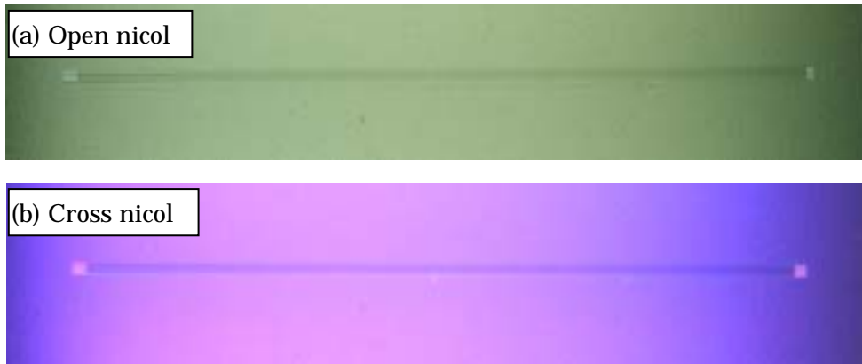
Fig. 9 Transmission polarized image of ceramic waveguide element from side view.
