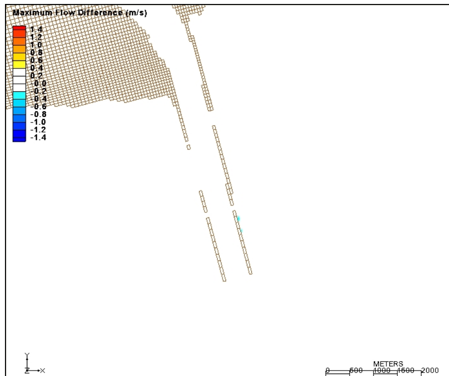
Figure B13. Difference in maximum flow magnitude between Plan 3 and existing conditions for the SW Storm in 2010.
