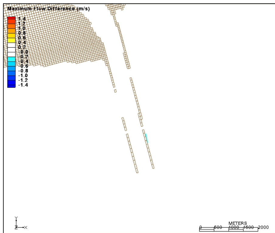
Figure B7. Difference in maximum flow magnitude between Plan 3 and existing conditions for the low-energy wave simulation in 2060.
