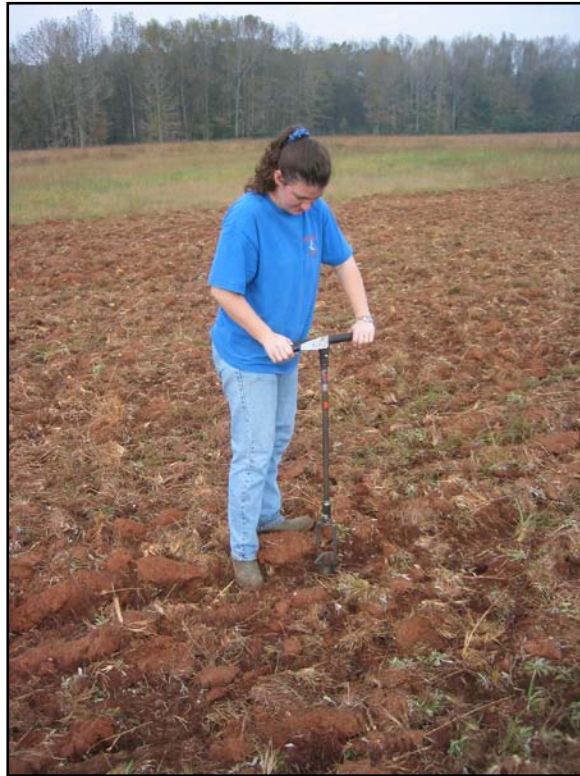
Figure 5. Taking a core from the soil surface.
