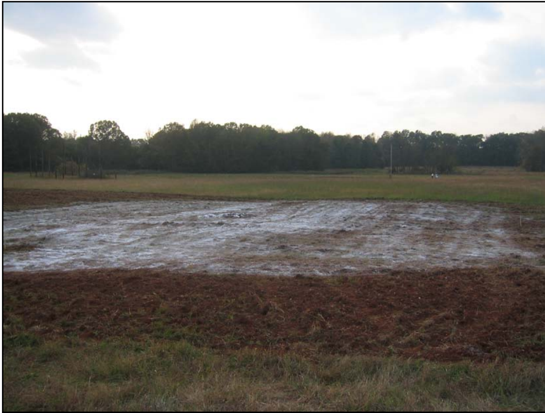
Figure 3. Site #4 after treatment with 227 kg of hydrated lime.
