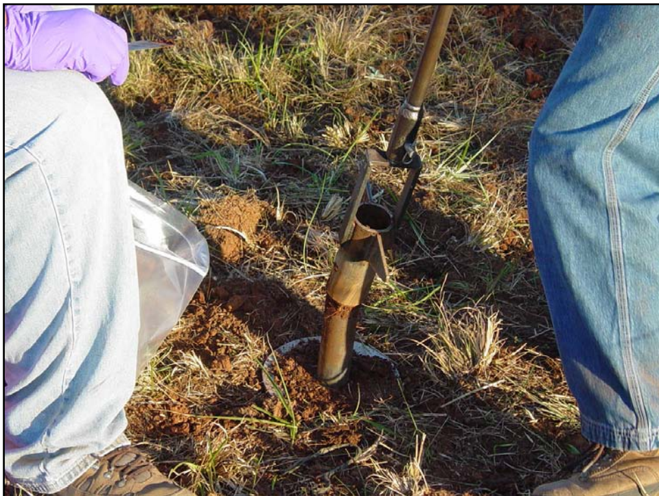
Figure 6. Pushing a soil core out of the tool.
