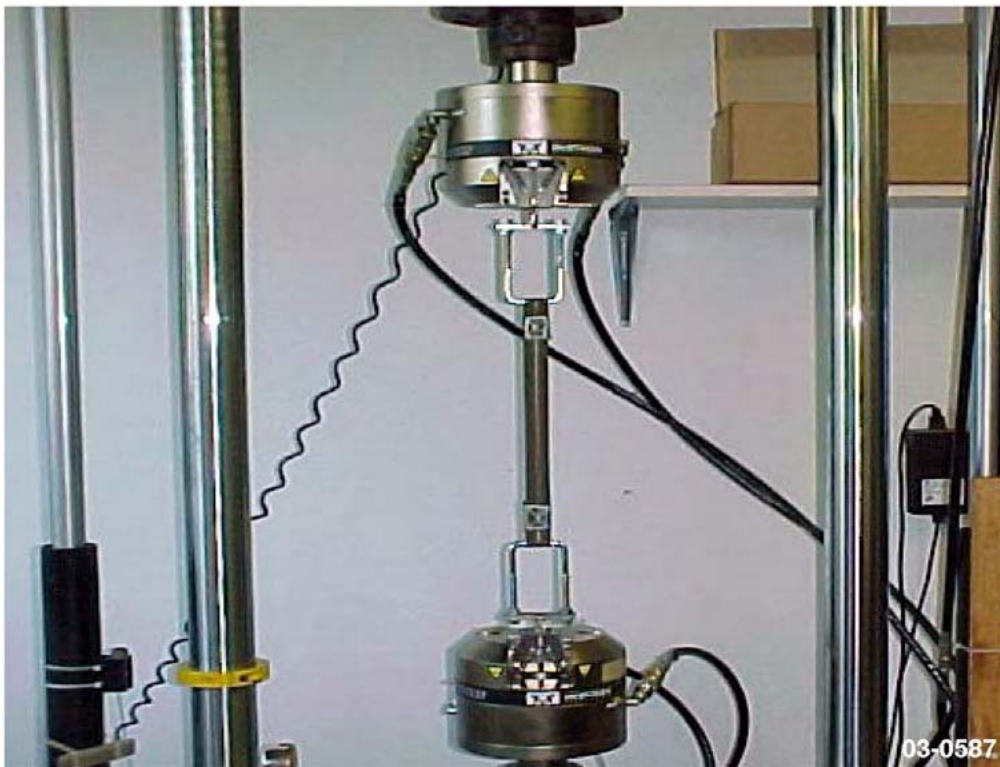
Figure 50. Tensile fatigue test setup
