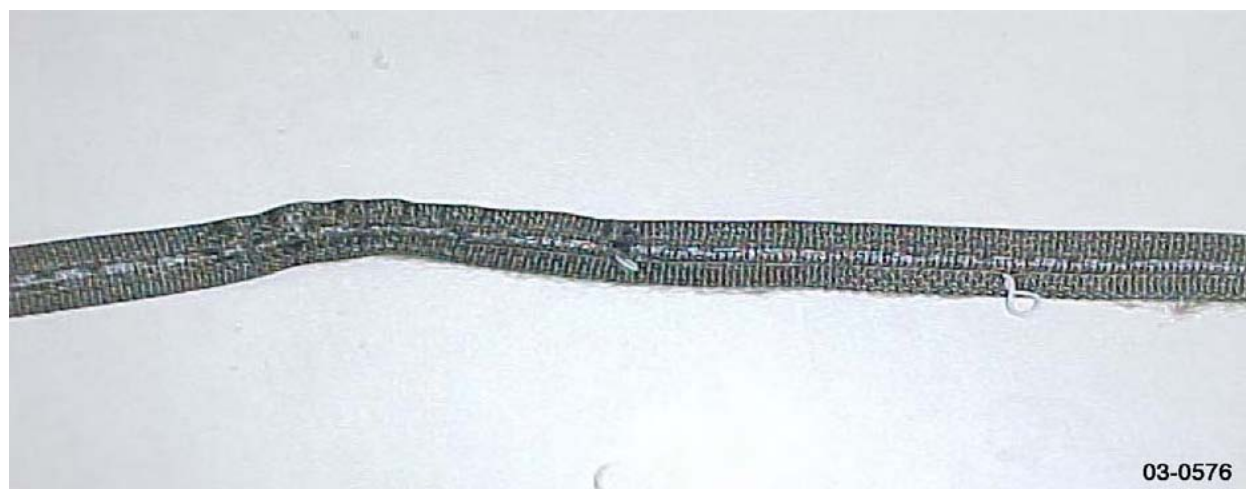
Figure 30. Effect of 2000 cycles of hex-abrasion testing USB v1 cable
