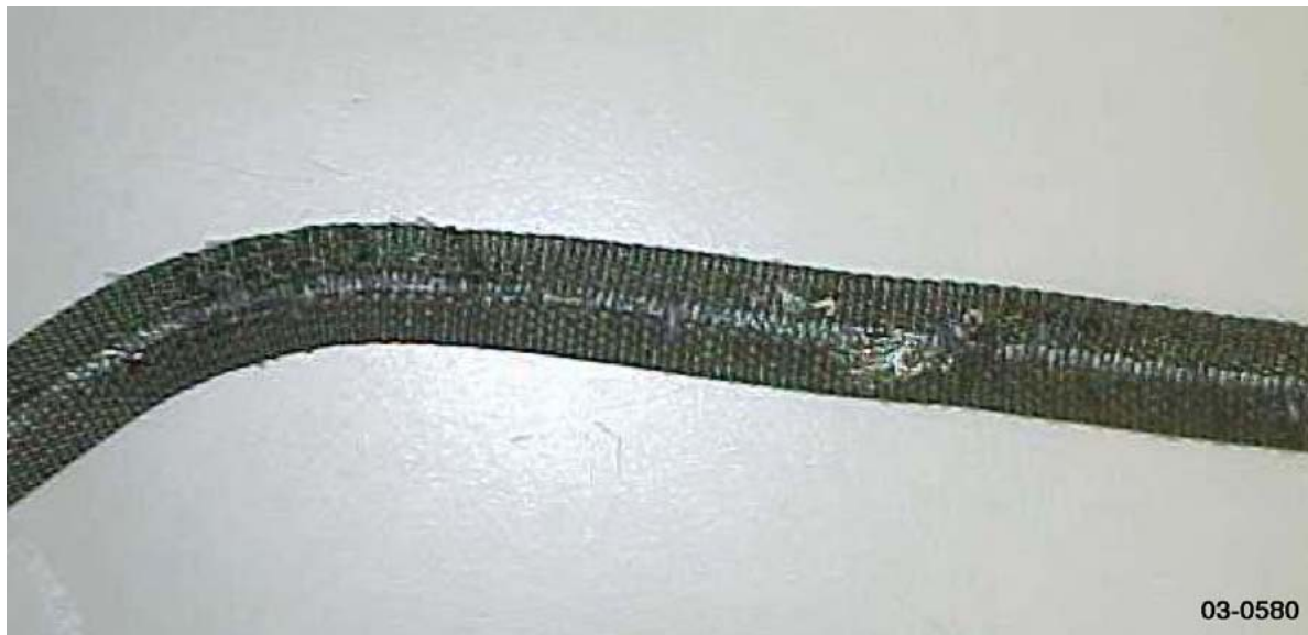
Figure 34. Effect of 2000 cycles of hex-abrasion testing on USB v2 cable
