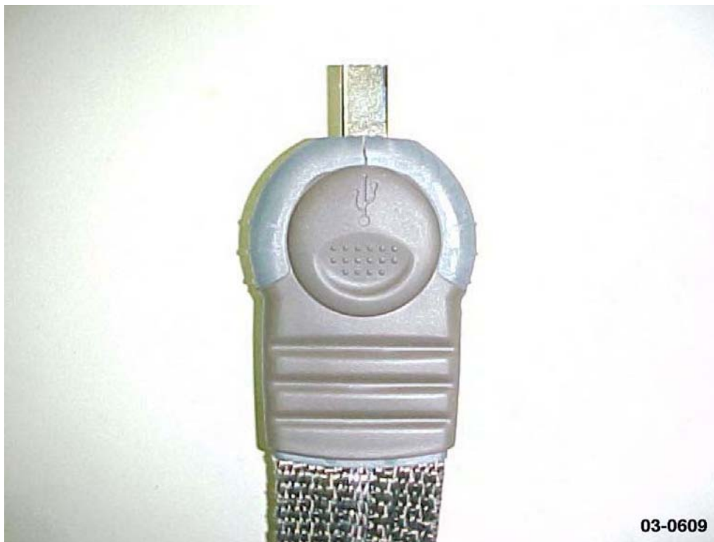
Figure 90. Cracking near USB plug
