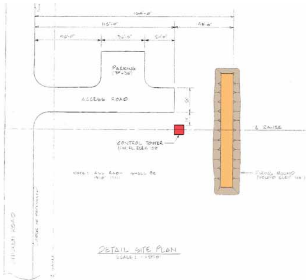
Figure 324. Transition firing range, machine gun range 53, Detail site plan, Fort Bragg, NC, 1978 (Standard drawing DFE-3278 sheet 6 of 10, Transition firing range, machine gun-range 53, range details, 19 January 1978).
