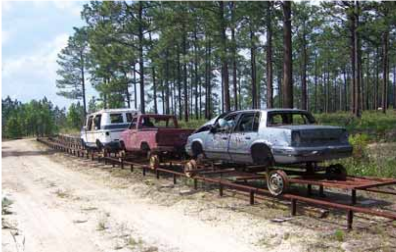
Figure 493. Target cars mounted on dollies and pulled by a cable system on a moving target track, Fort Bragg, NC, 17 May 2006.
