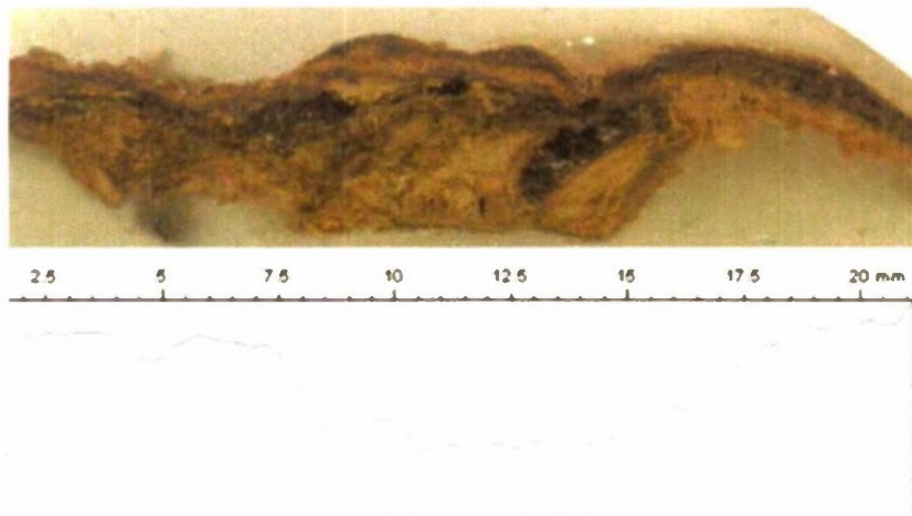
Figure 3. Cross section of tubercle and profile of pitting associated with DSH tubercle.
