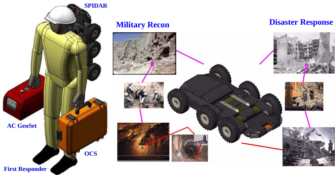
Figure 20 : Deployment of SPIDAR by a single person into multiple civil-defense/military missions
