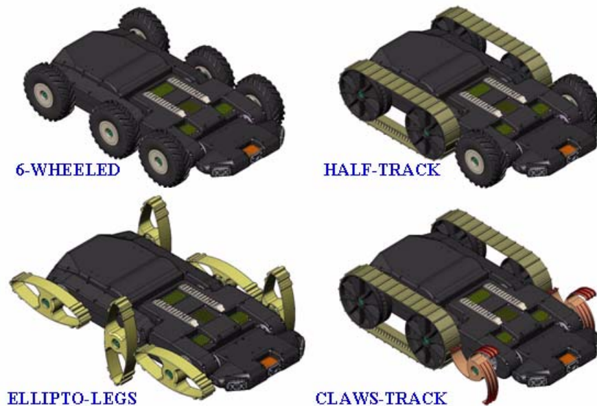
Figure 10 : Possible running-gear configurations for SPIDAR
