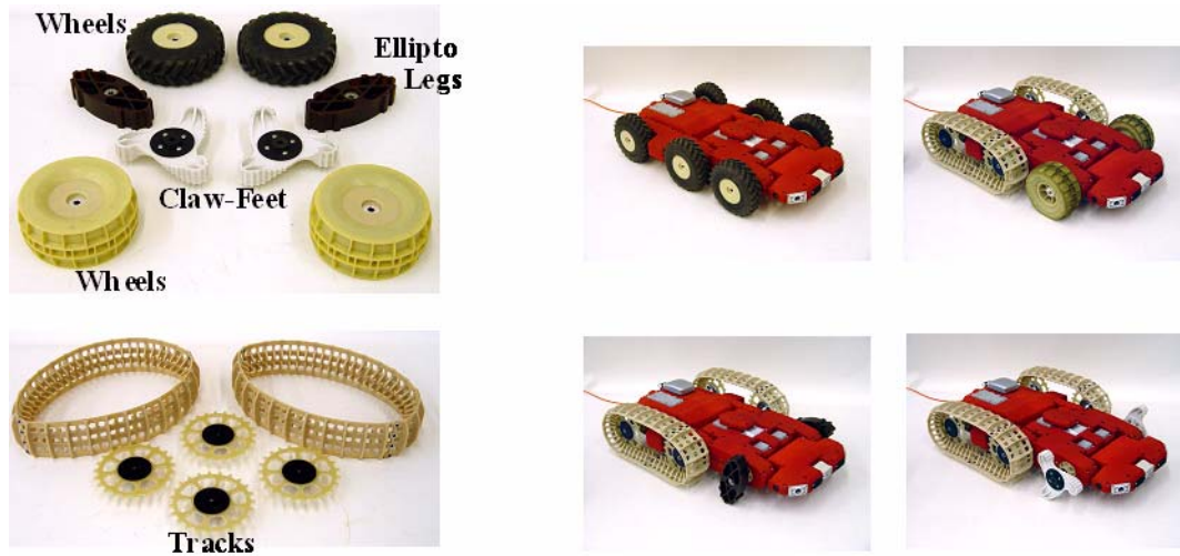
Figure 25 : Varied locomotion configurations
