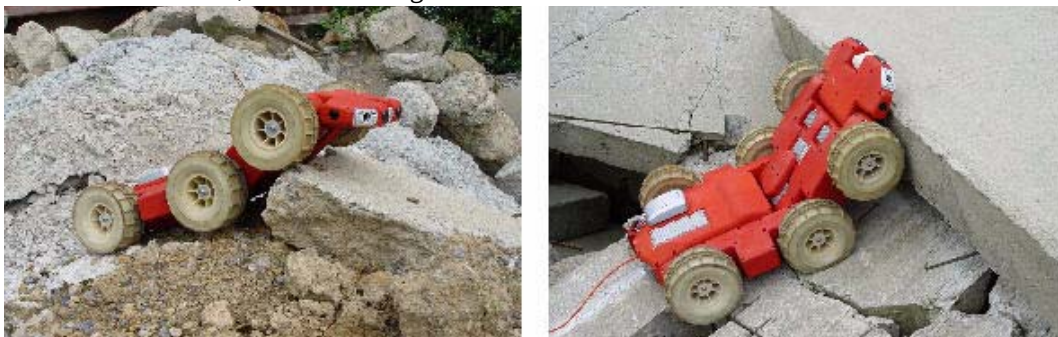
Figure 30 : SPIDAR prototype articulating its chassis/abdomen and sensor head for better inspection and a climbing attempt
