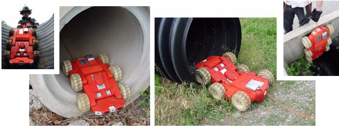
Figure 33 : SPIDAR driving out-of a concrete sewer-main and into an exposed corrugated drainage pipe
