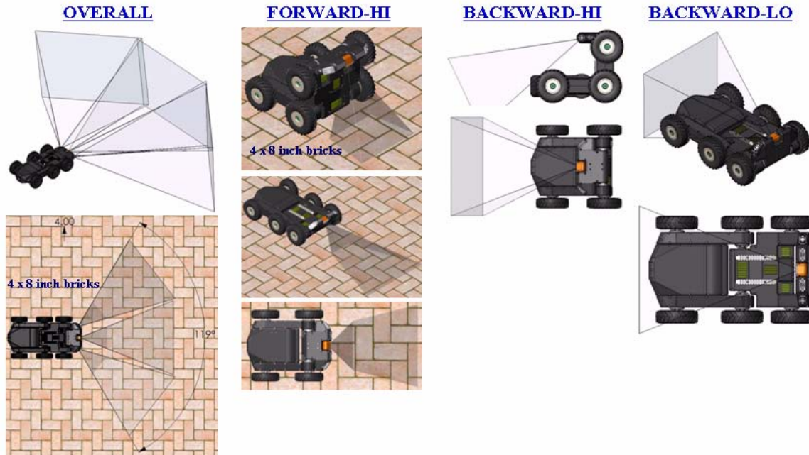
Figure 6 : SPIDAR robot platform FOV configurations for forward camera(s)
