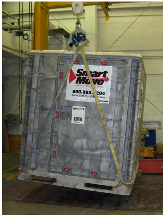
Figure 28. Rotational cornerwise drop test, -30°F.
