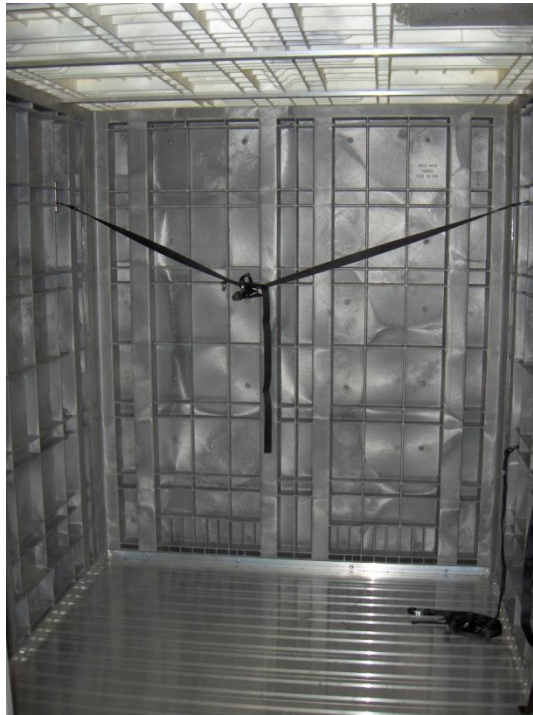
Figure 3. Container interior, showing molded walls and aluminum floor.
