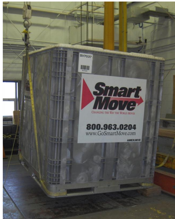
Figure 22. Rotational cornerwise drop, ambient.
