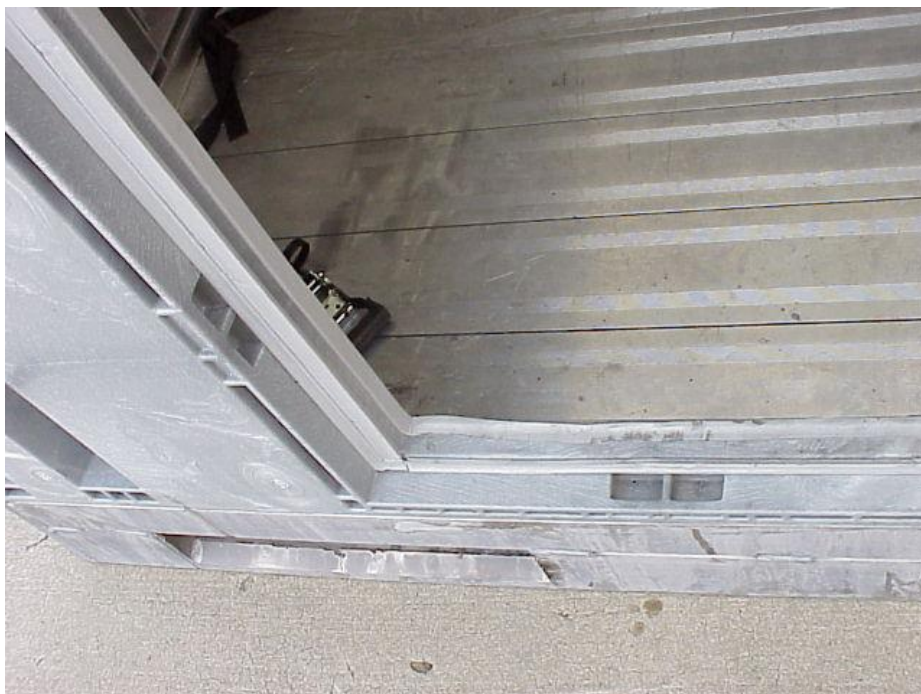
Figure 12. Latching side door gaskets, bottom corner.
