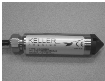
Fig.2.1: Photo of Pressure Sensor.
