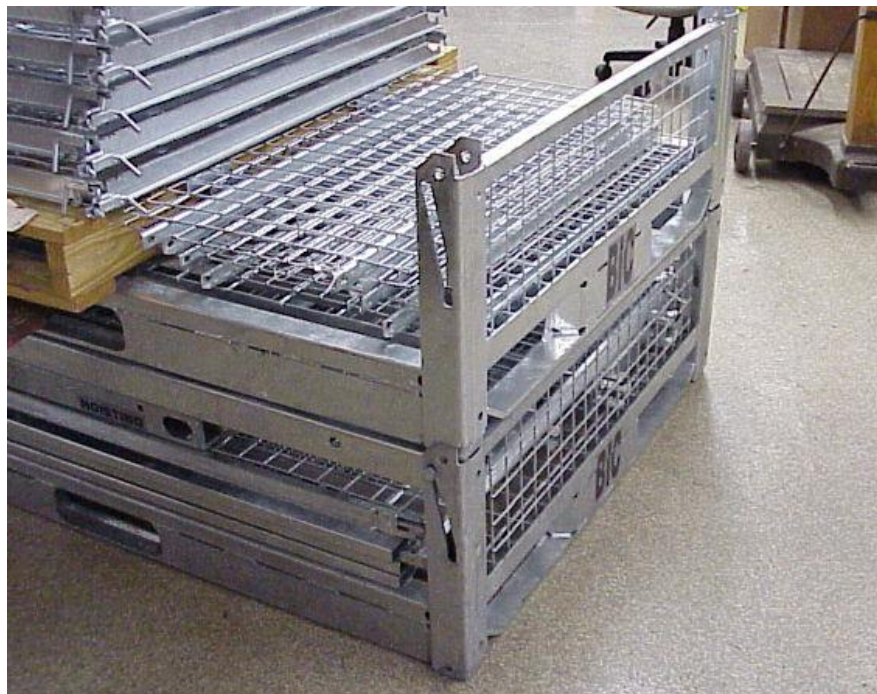
Figure 6. Stacking interface of two collapsed CCPs.
