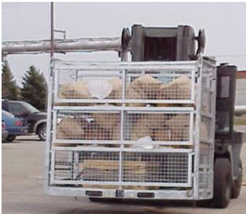
Figure 26. Vibration test method (transport over rough roads).
