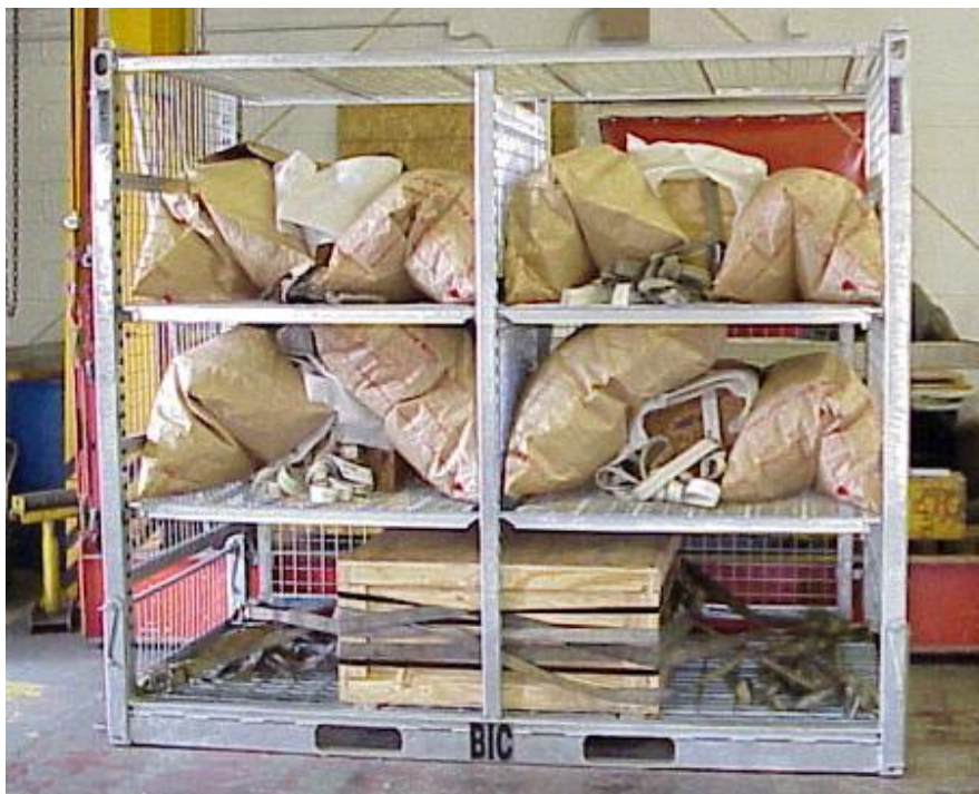
Figure 14. Placement of test loads.
