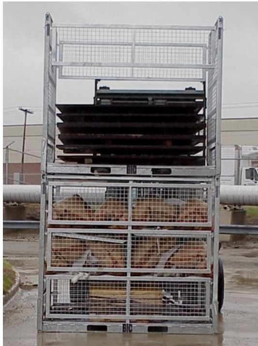
Figure 29. Superimposed load test.
