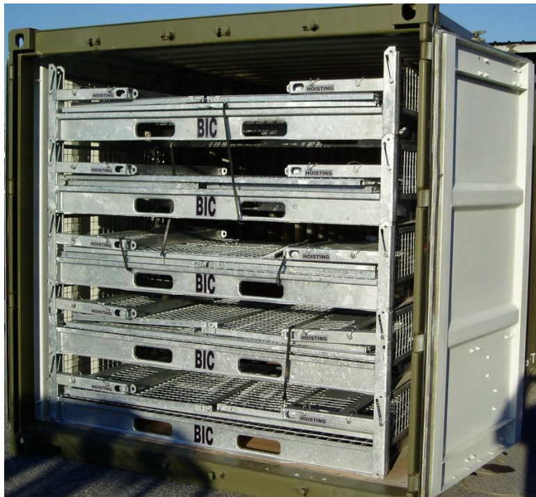
Figure 7. Collapsed stack of 5 VCP pallets (same collapsed (calculated) height as 5 CCPs) in ISO container (at BIC).
