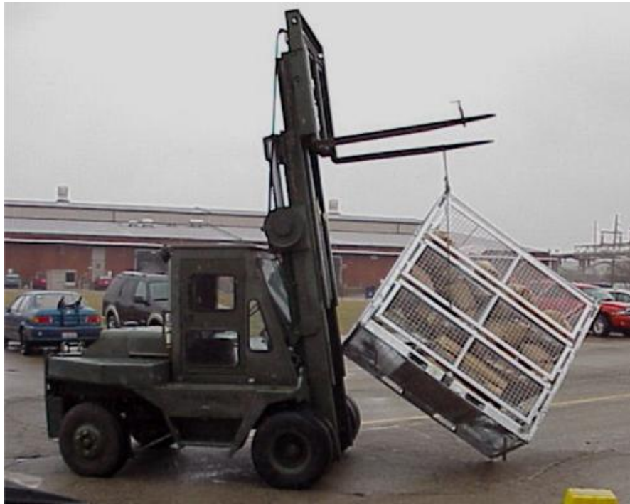
Figure 25. Single hoist fittings strength test.
