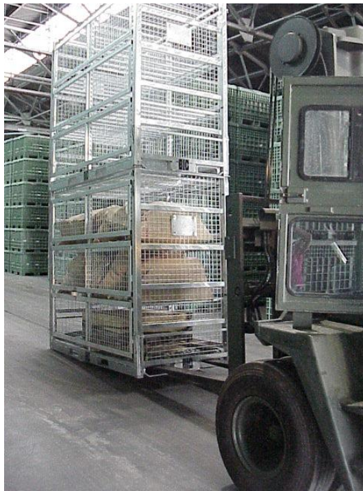
Figure 23. Forklift truck handling test, lifted push.
