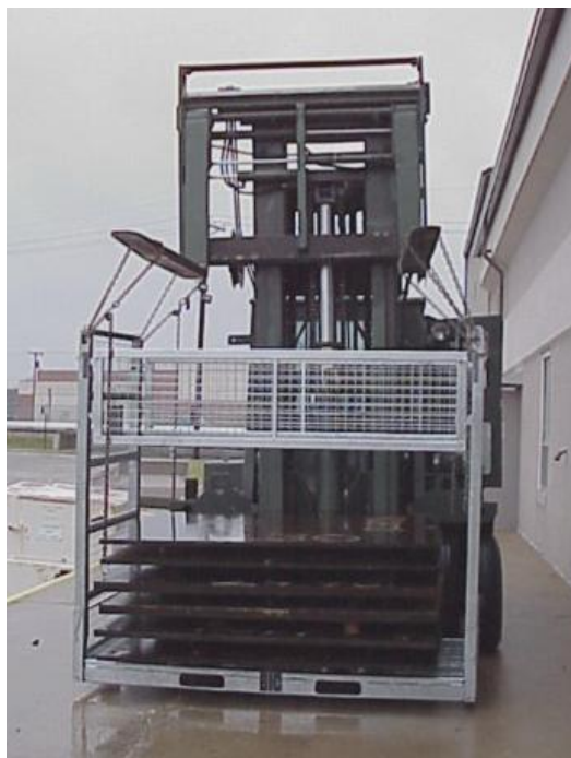
Figure 28. Hoisting fittings strength test.
