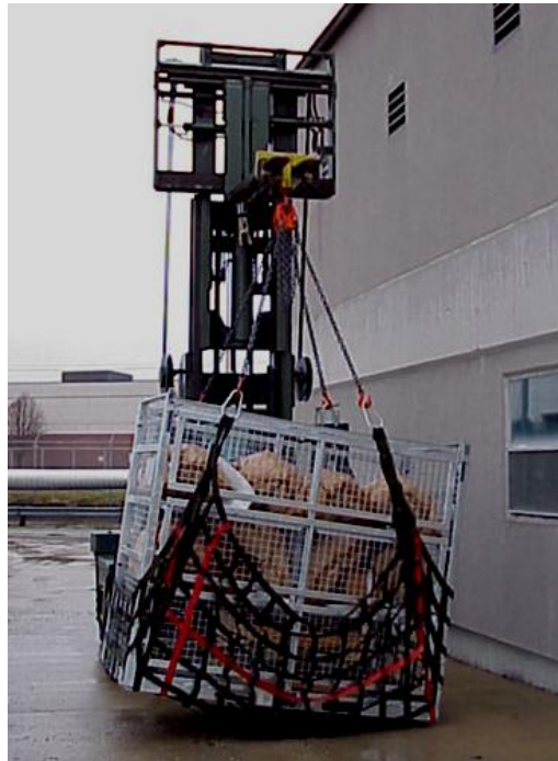
Figure 27. Sling handling with cargo net.
