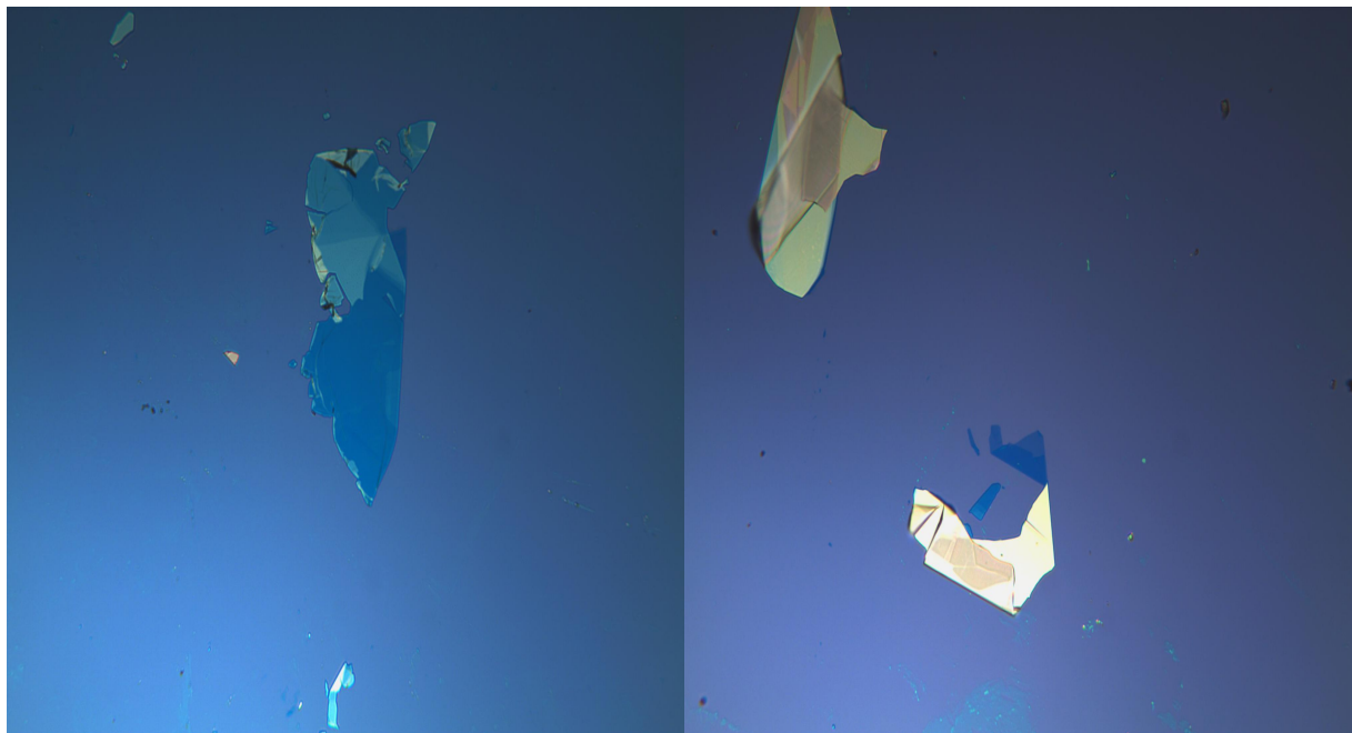
Figure 7. Optical micrographs of two areas on 300 nm of SiO 2 with graphene and graphite present. The yellow areas indicate the presence of thick, multilayer graphite, while the blue areas indicate few-layer and even monolayer graphene.
