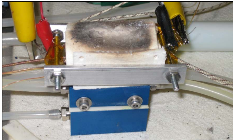
Figure 16. Fully assembled test fixture with cartridge heaters inserted.
