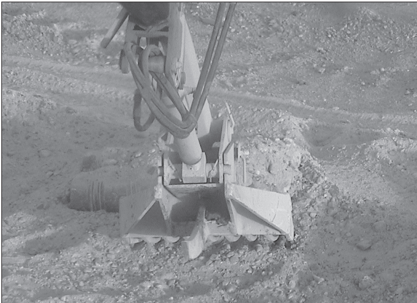
A Buffalo arm investigates an IED buried on the shoulder of a road.
