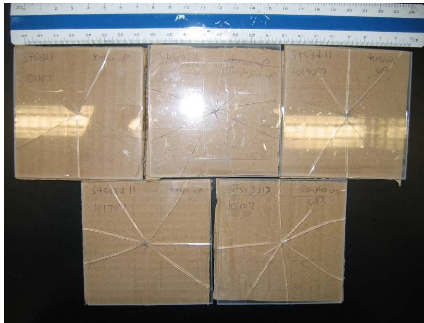
Figure 32. Several failed 3.2-mm Starphire tiles. The star-like fracture patterns are typical of biaxial flexural testing. Top row, left to right: 0.125-, 0.25-, and 0.5-in ball. Bottom row, left to right: 0.5-in ball and only bottom surface abraded, 0.0625-in ball. Tiles are 4 \times 4 \text{ in}^2 .
