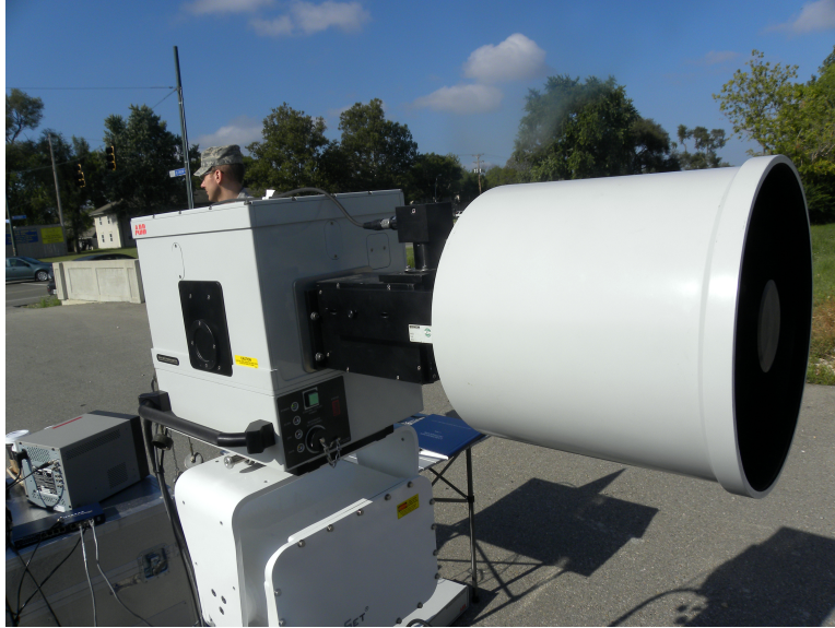
Figure 15. Picture of the Bomem MR-304 with attached 4.9 mrad Cassegrain telescope. This picture shows the MR-304 mounted on a Quickset gimbal for sensor pointing and target acquisition. This was the setup used for the Smoky SAM test.
