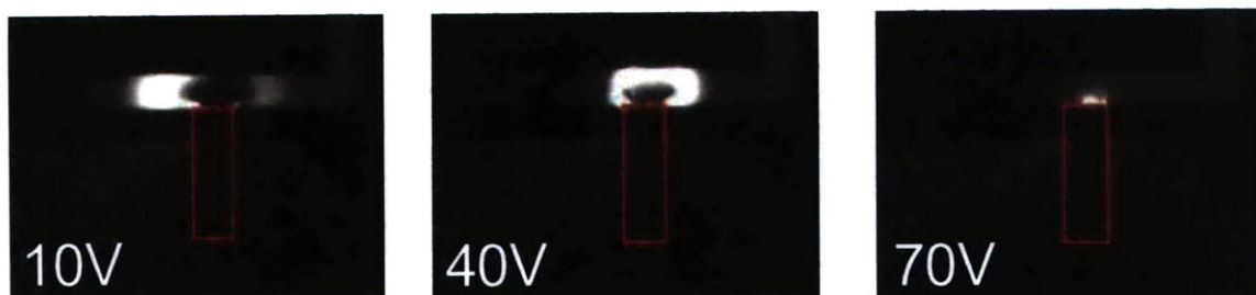
Figure 6-13: Concentration polarization behavior of third generation integrated devices. The voltage applied across the nanochannels is overlaid and the location of the nanochannel filter outlined in red. Although no voltage was applied between the termini of the anodic microchannel, the depletion region was self-stabilizing, indicating EOF through the filter.
