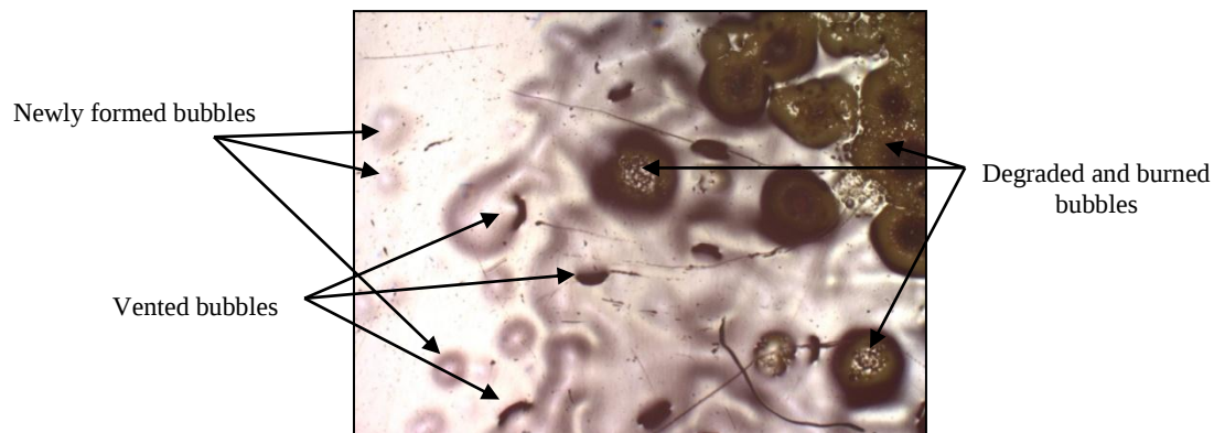
Figure 27. Paint sample showing stages of thermal degradation
