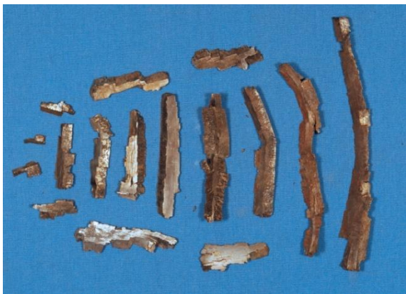
Figure 13. A portion of the fragments recovered from the ES-1 plane strain condition experiment
