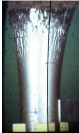
Figure 14. Optical image of expanding ES-1 steel cylinder
