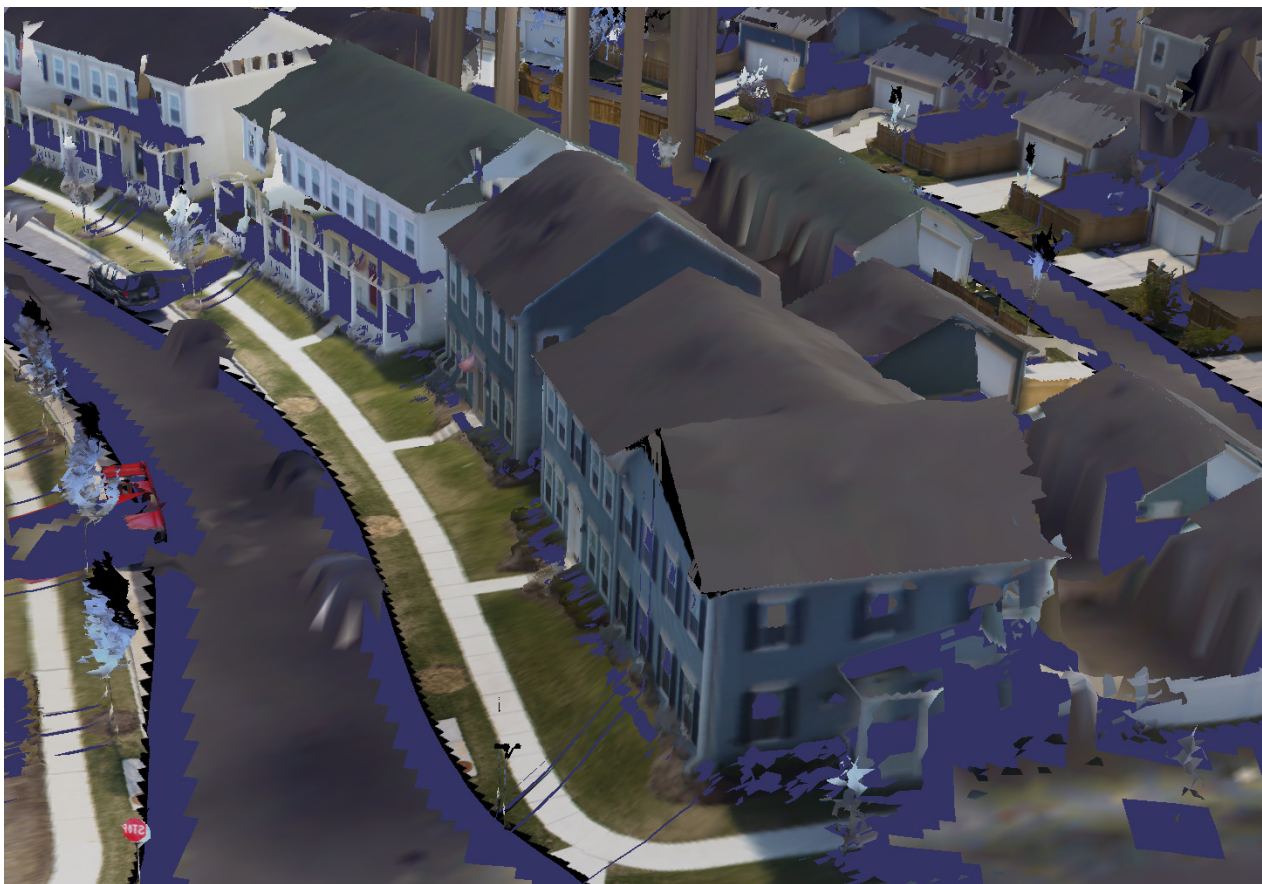
Figure 6. The dense terrestrial mesh is merged with a coarser airborne mesh.
