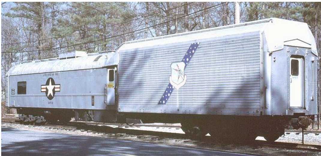
Figure 4. KC-135A Instrument Flight Trainer Railroad Car. 3
