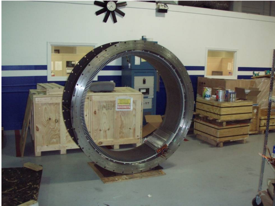
Figure 5: Stator for Beta TGU permanent magnet generator being wound
