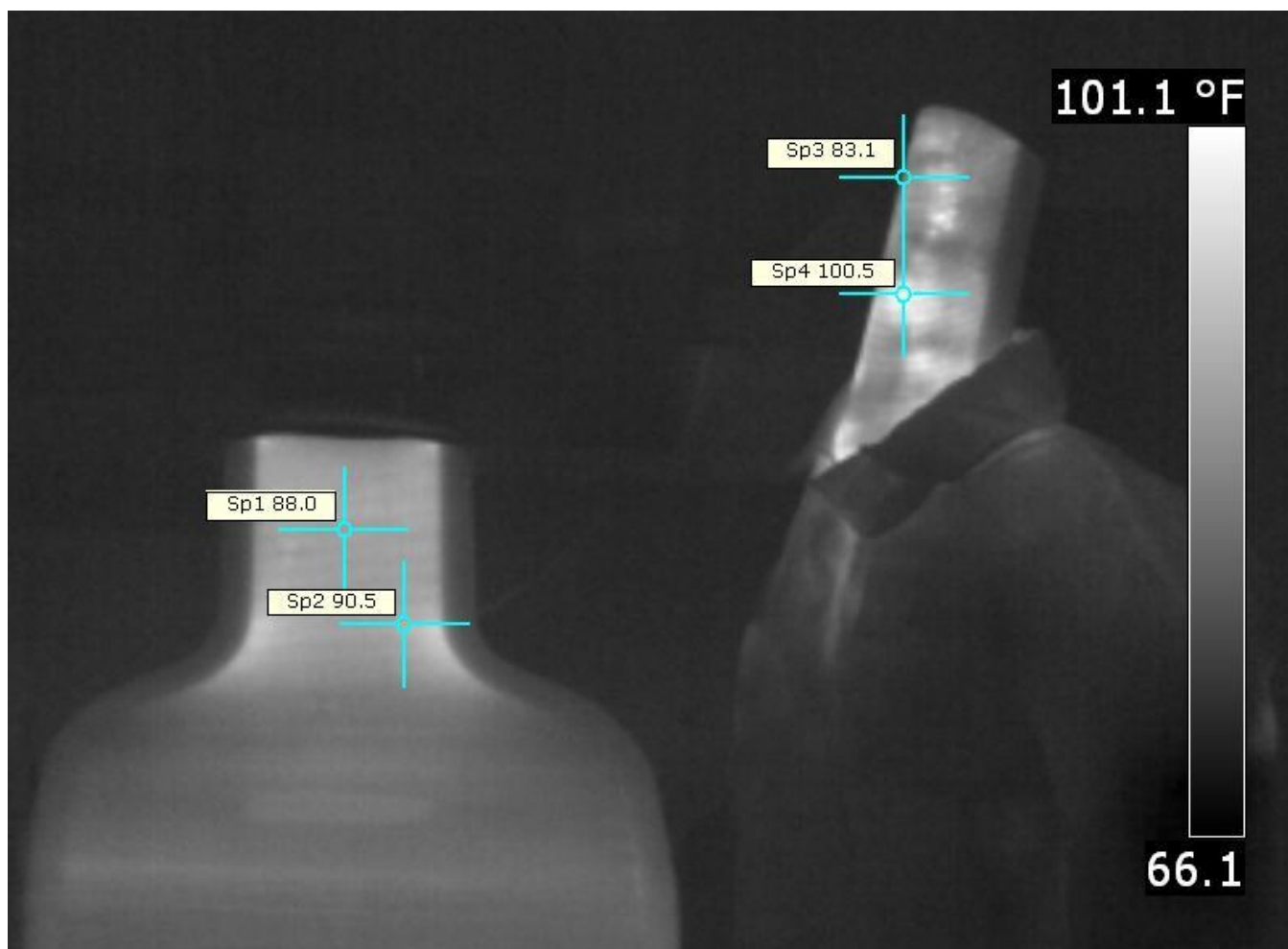
Figure 18. GTT target comparison- new and post-test (Note non-uniformity of the Post Test Target due to damaged wire mesh).
