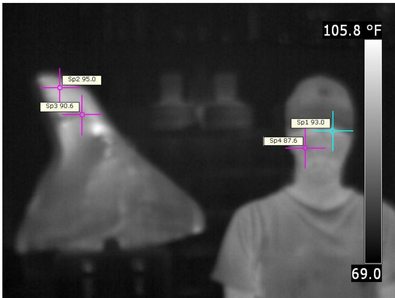
Figure 14. GTT OSCAR target repair testing compared with a human, CG Station Sand Key.
