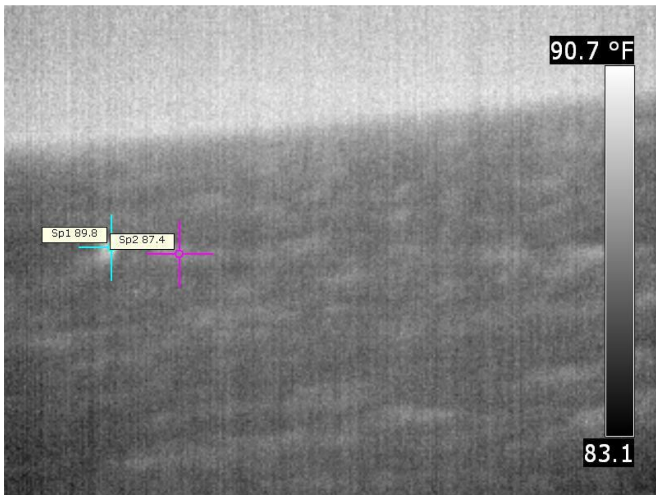
Figure 11. Thermal infrared image of the GTT Oscar is shown from the first night of testing. The temperature difference was 2.4 degrees Fahrenheit between the GTT Oscar and the maximum sea water temperature created from thermal clutter due to whitecaps.
