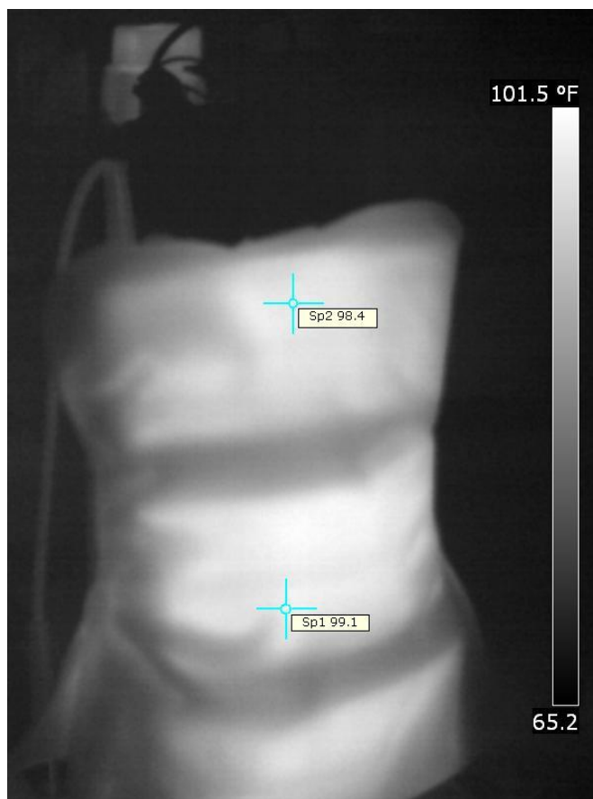
Figure 2. HDV prototype thermal testing is displayed, shown with the head unit only (front profile).
