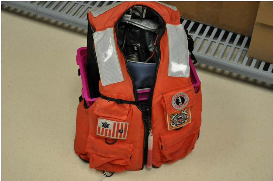
Figure A-12. An upper-forward tie-strap connection of the PFD is made to the crate.
