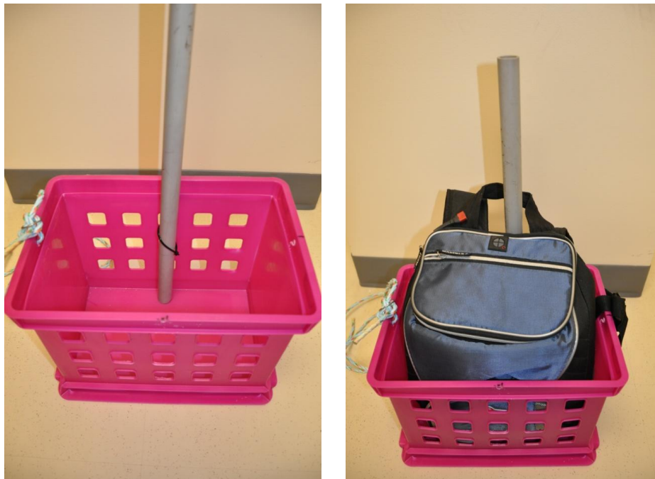
Figure A-10. PVC pipe installed in crate, and with the bag unit inside the crate.
