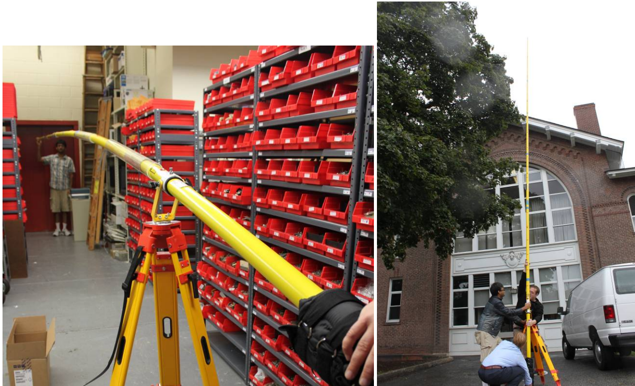
Fig. 16. Left - telescopic pole in the ECE shop with partially assembled coaxial antennas; right - telescopic pole in its full length and in the vertical position with most of antennas removed.
