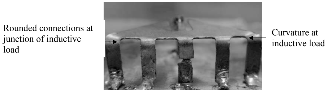
Figure 11. Picture of fabricated antenna indicating rounded connections and curvature at junction between antenna top sector and inductive loads.
