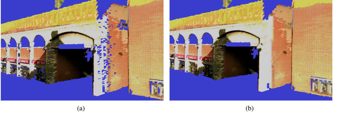
Figure 12: Mesh (a) with holes and (b) with holes filled. The point clouds used to generate these meshes are not from S1 or S2. Instead, they are from a dataset which was obtained using multiple sensor passes.
