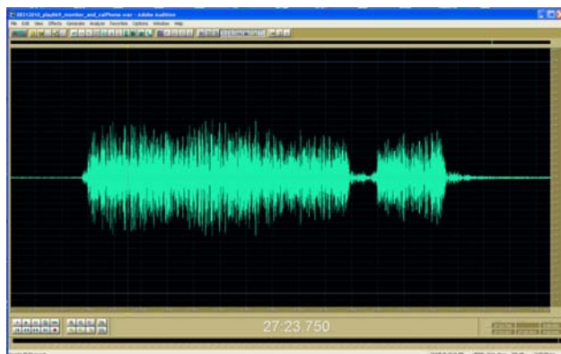
PRN time domain (waveform) representation
