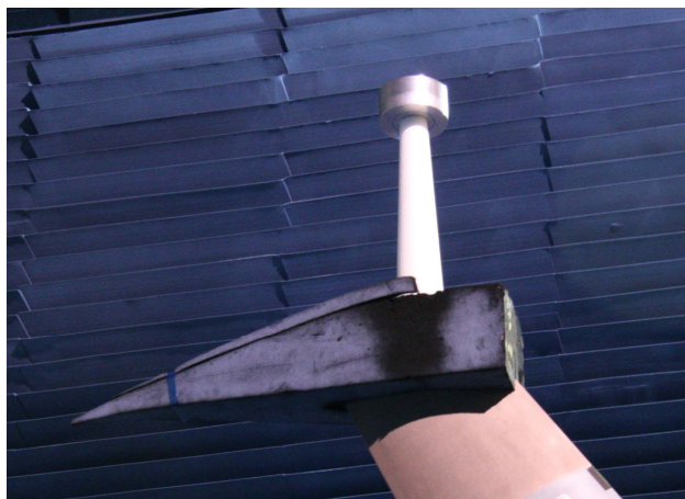
Figure 8. Calibration Target on the Pylon Rotator
