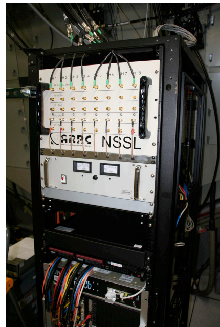
Figure 2: Picture of the recently installed system. The top section contains the eight RF to IF downconverters, while the bottom section contains the eight digital receivers.
