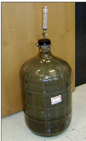
Figure 3-11. Macrocosm in 5-Gallon Carboy
