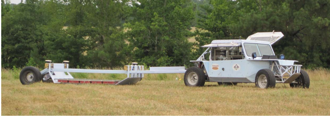
Figure 5-2 – MTADS tow vehicle and TEMTADS array.
