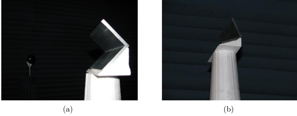
Figure 2.6. Dihedral targets for bistatic RCS measurements. (a) 90° roll and 45° pitch, with bistatic receiver in background. (b) 90° roll and 20° pitch positioned on pedestal. Orientations are relative to the original dihedral position defined in Figure 3.3.
