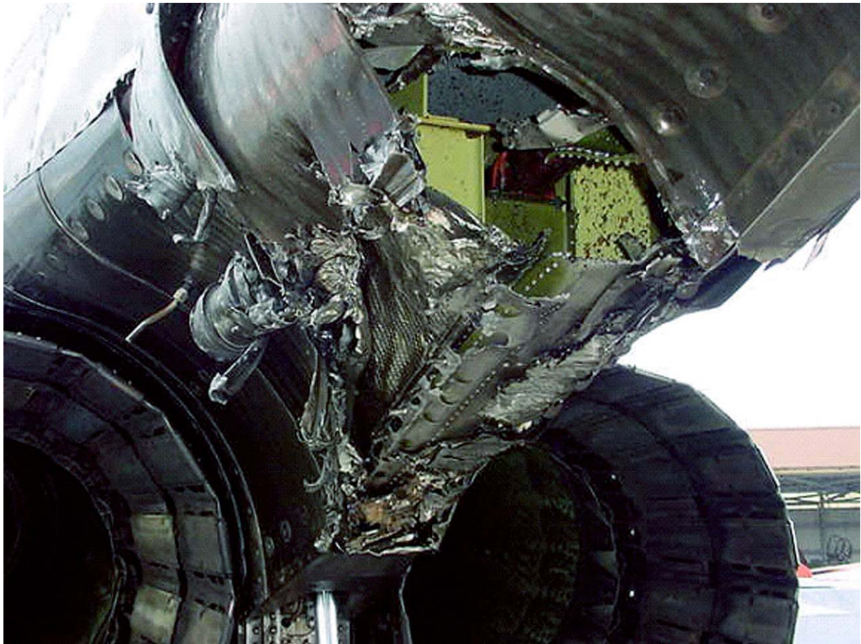
Figure 1-5: F-4 Empennage Battle Damage, courtesy of USAF [5]
