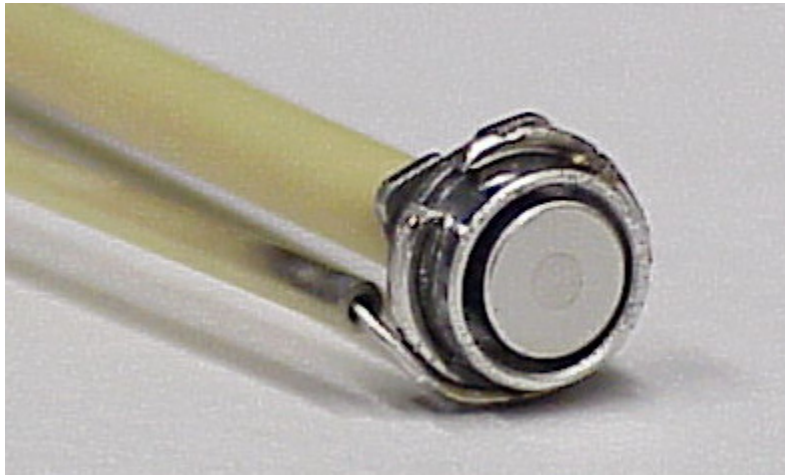
Figure 12: Nude Faraday probe with casing removed, taken from Azziz et al. [17]
