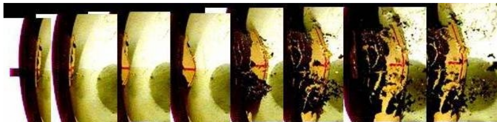
Figure 1. Dynamic (increasing time left to right) development of helmet back-face deformation.
