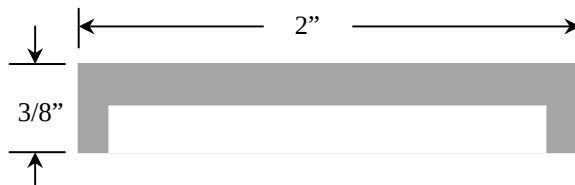
Figure 28. Cartoon of obstacle structure for cross-over obstacle and leading obstacle on the top of Tube 2.
