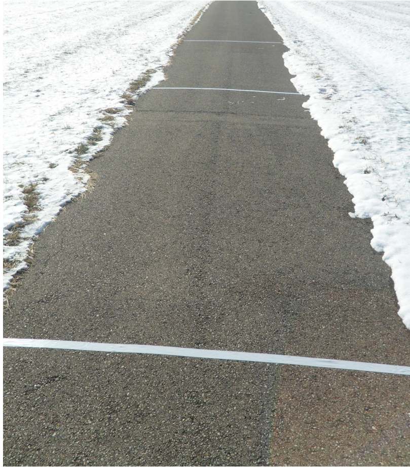
Figure 3.11: Ingressing track setup where the lines correspond to zero, five, and ten meters.
