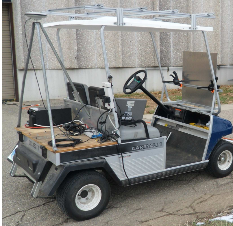
Figure 3.9: The AFIT Advance Navigation Technology (ANT) Center golf cart equipped with differential GPS for enhanced precision navigation and timing.
