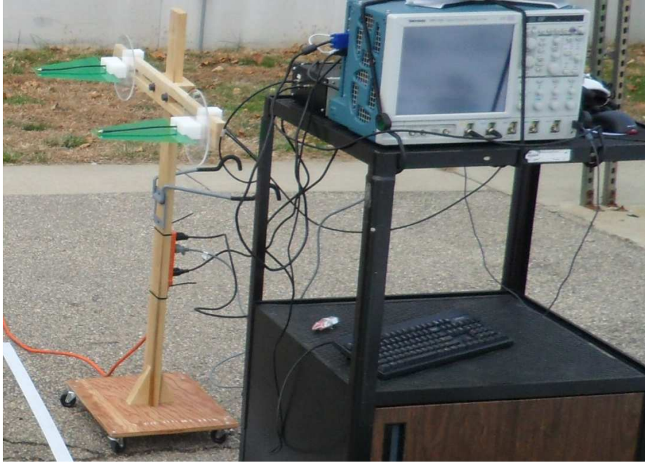
Figure 3.10: The antenna stand connected to the radar box (black box behind oscilloscope), which is connected to the Tektronix DPO 7254.
