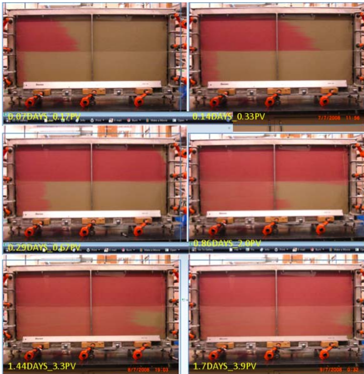
Figure 5-1: Photo results of amaranth dye tracer test (no polymer addition) within tank 2L_50%UNI30_50%UNI70. Top layer is the higher-permeability sand.
