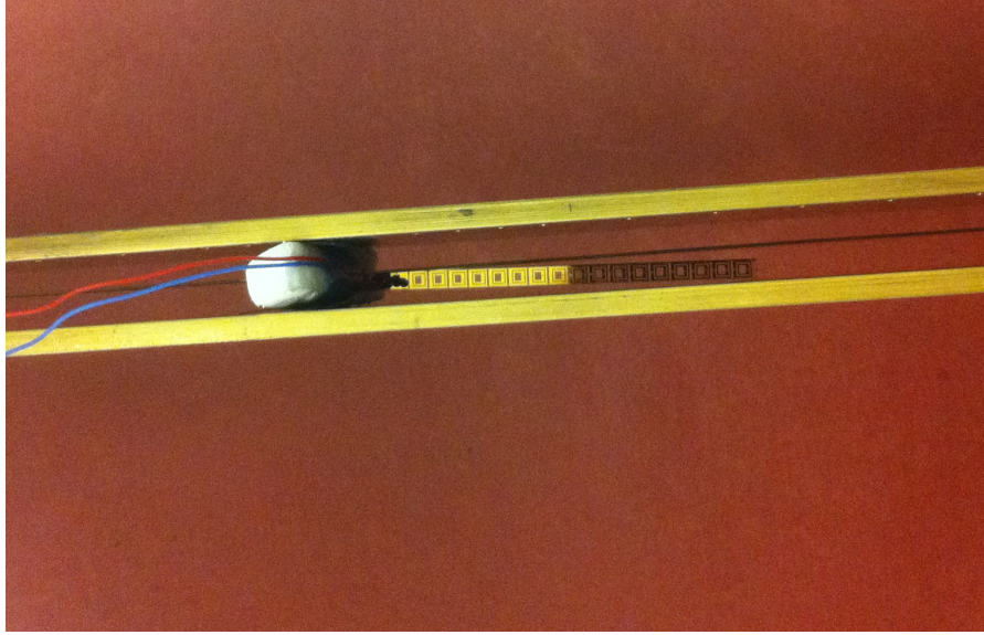
Figure 85. Experiment setup for stripline measurements of the 10 GHz AFIT meta-material structures in the 18 GHz stripline.
