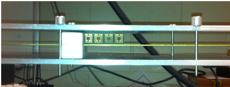
Figure 100. Experiment setup for stripline measurements of the 3 GHz AFIT metamaterial structures in the 4 GHz stripline.
