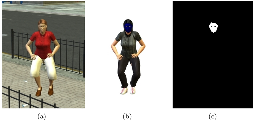
Figure 18. (a) An original image patch. (b) A “blue masked” version of the same dismount and pose as in the image patch. (c) The application of Eqn. 17 effectively identifies the head skin island.
