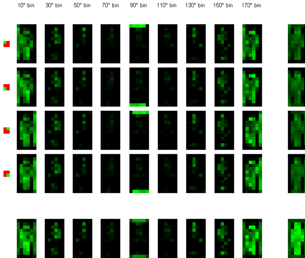
Figure 17. Spatial mapping of a HOG feature divided into orientation bins across the top and originating block position down the left. The block position for each row is indicated on the left as a green square occupying one of four positions on a red background. In the remainder of the figure, brighter shades of green corresponds to larger values. For simplicity in viewing, the 36 frames can be averaged across orientation angle (far right column) or originating block position (bottom row). The bottom right frame displays an averaged cell magnitude representation of the dismount.
