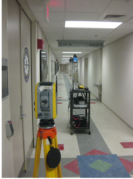
Figure 4.16: Experiment Setup with LD-OEM 1000 Laser Scanner Mounted on Cart with Trimble S6 Surveying System in the Foreground
