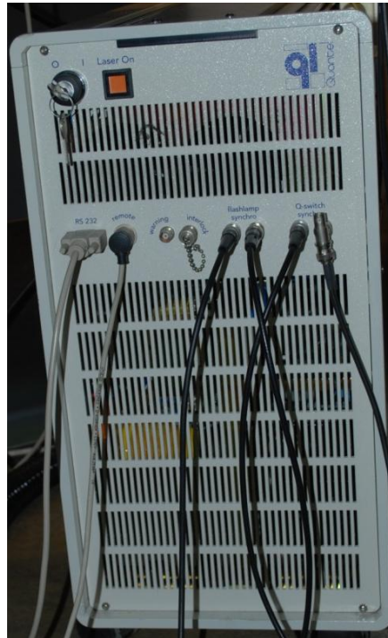
Figure 14. Power Supply and Cooling Group Unit
