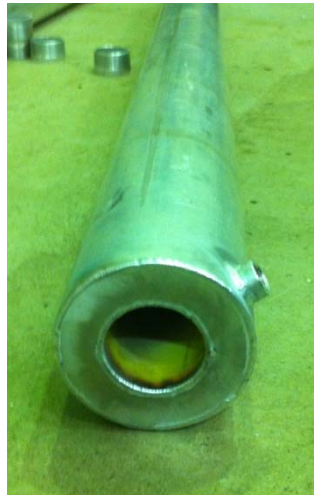
Figure III-1: Aluminum heat exchanger section before addition of pipe nipple
