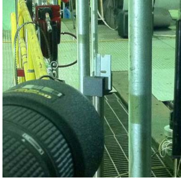
Figure III-16: Phantom camera aimed at vertical knife (razor blade) edge
