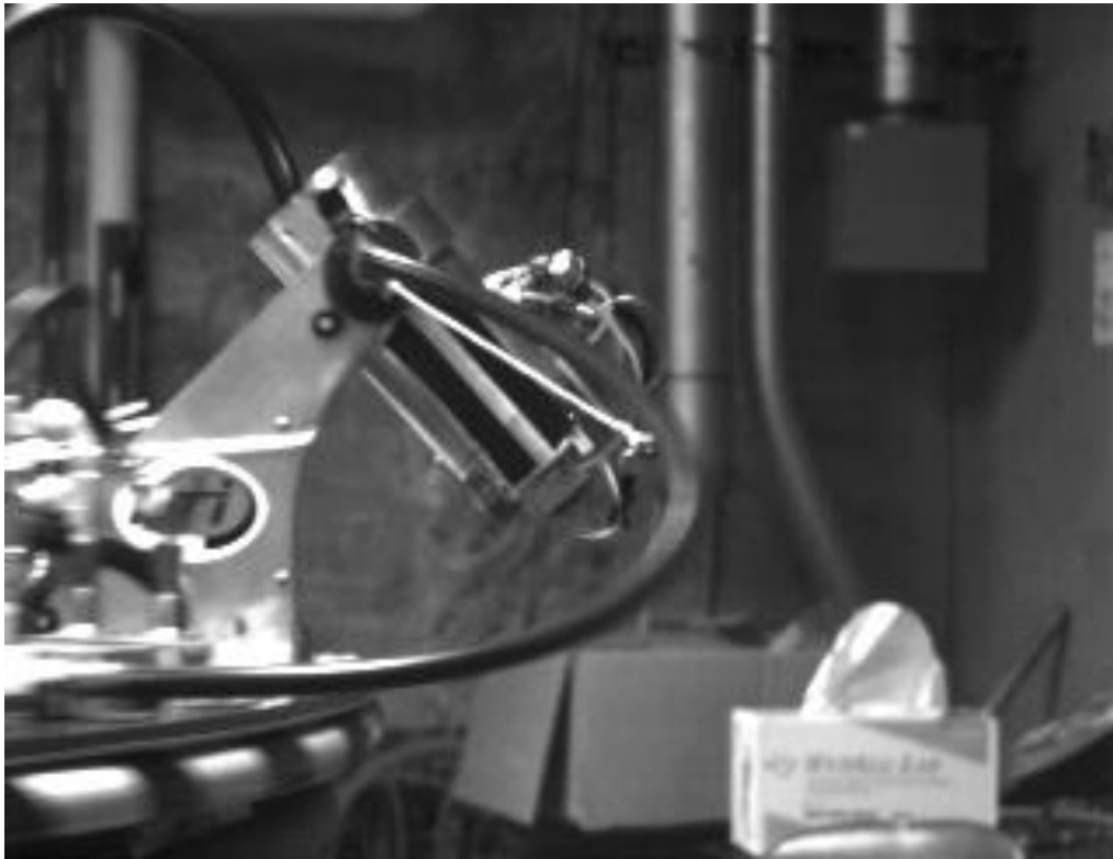
Figure 3: Acceleration Vector Error Experiment. The Plumb-Bob (White String) Angle Is Shown In Relation To The Angle Of The Reservoir In The 2g Test Case
