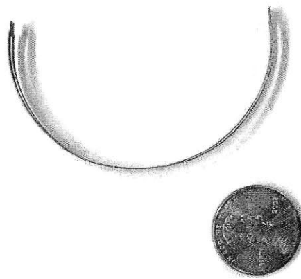
Figure 4.6: Flexure beam is curved around 9mm diameter cylinder, to preload the flexure. The preload propels the mechanism forward when the string is released.
