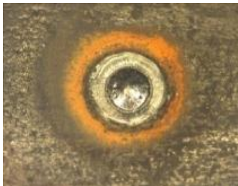
Fig. 9 Molten pool on a heat exchanger tube
